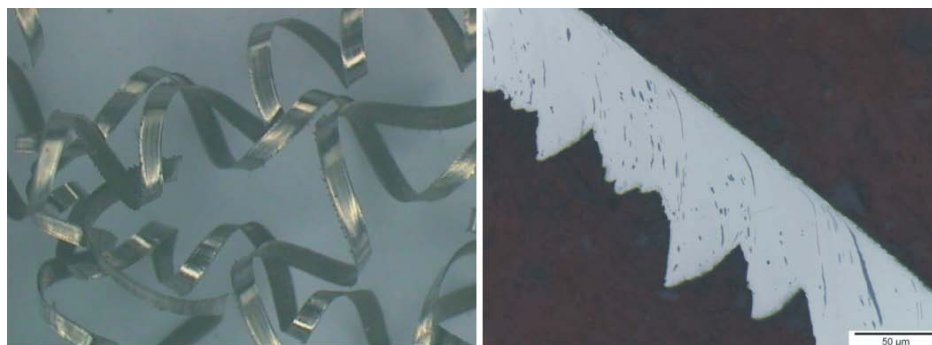
Figure 8. Chips obtained during life test with the steel with the addition of Ca. Bar scale 50μm.
