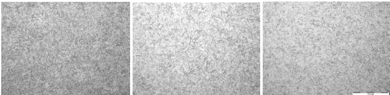
Figure 7: Region D microstructure: a) HI = 0.5 kJ/mm; b) HI = 1.5 kJ/mm and c) HI = 2.8 kJ/mm.
