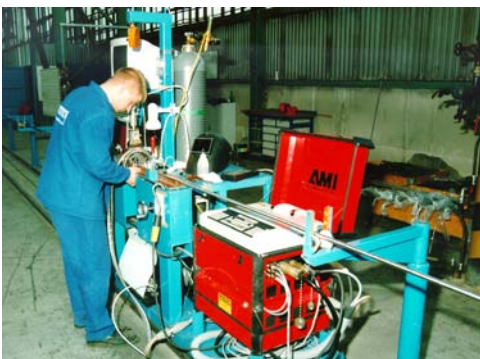
Figure 2. Left: Sandvik orbital welding set-up with orbital welding power supply with cooling unit and orbital weld head. Orbitally welded lengths of super duplex tubing were wound onto large coils for umbilical tubing. 100% radiography of the orbital welds was performed. (Photos from Henon, B.K., 2001)
