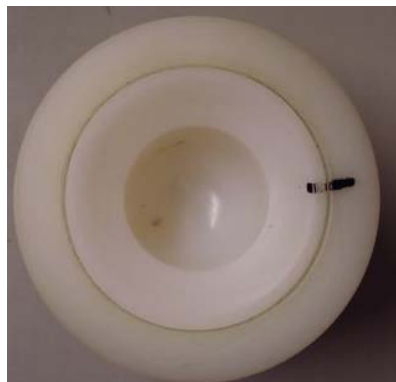
Figure 6. Surface of acetabular component after the test.
