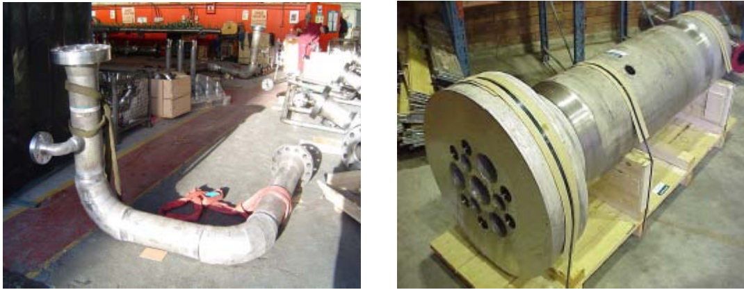
Figure 4 – a) A manifold part fabricated by HIP. b) A swivel fabricated by HIP.
