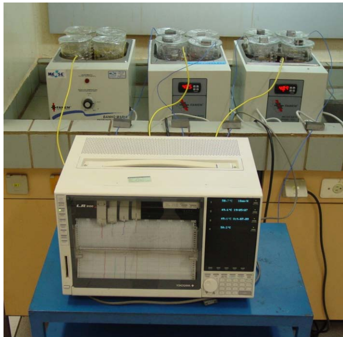
Figure 1- Apparatus for determination of pitting resistance according ASTM G-48 method A, showing the temperature recorder of the control thermocouples.
