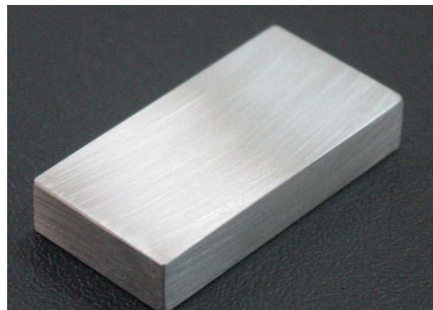
Figure 12 – G-48 corrosion specimen of the rebalanced steel after 24 h at 50°C showing no pits on the testing surface.
