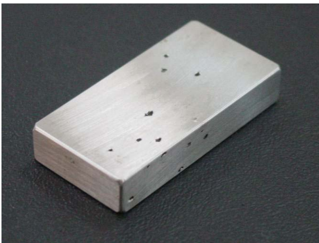
Figure 4 - Conventional steel corrosion surface of the G 48 specimen 606 after 24 h at 50°C showing the pits.
